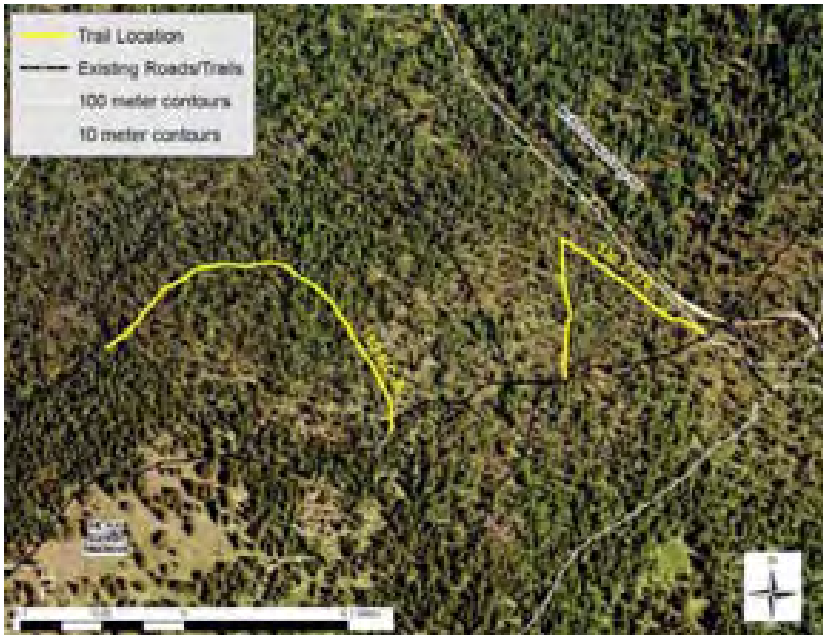
Figure 31. Map depicting the location of proposed trail 160 KC-A (on left). Trail 160 KC-A is proposed to be constructed around the east- to north-facing slopes of Mt. Kit Carson, just west of the proposed Trail 130 / 170 (Figure 31). The purpose of this proposed trail is to reduce the trail gradient of the existing trails, thereby reducing erosion issues and improving access conditions for a host of user groups including more novice mountain bikers. As can be seen in Figure 32, the proposed trail goes mostly through a forest of subalpine fir / common beargrass (S3 G5), with a small patch of subalpine fir / thinleaf huckleberry encountered on the eastern flank of the mountain (S4 G4). The forest on the eastern flank was formerly dominated by lodgepole pine that is now naturally dying off and being replaced by younger subalpine firs in the forest understory. Table 12 describes the plant associations and their relative abundance along the proposed trail route.
