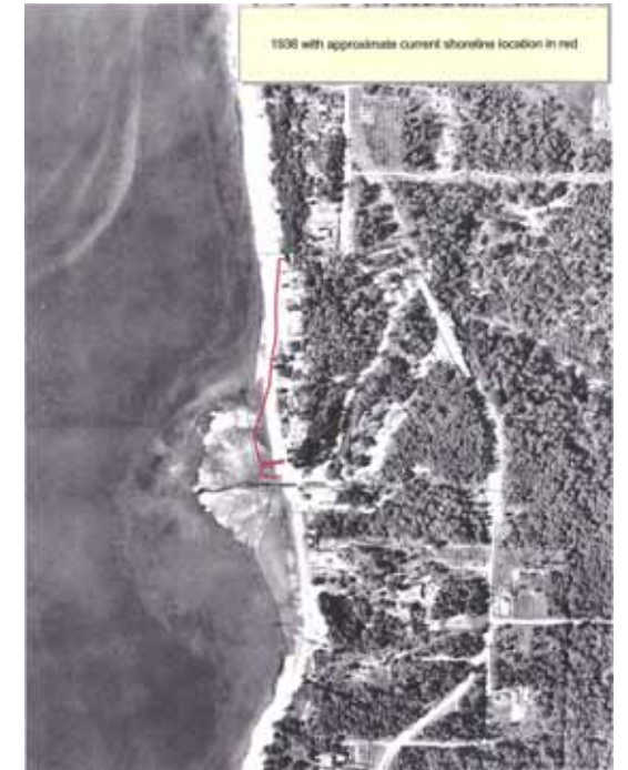
1936 Aerial Photo and current shoreline configuration (red line). Note that McSorley Creek historically enters Puget Sound further south and shoreline has been filled to extend shoreline waterward from historic configuration.
