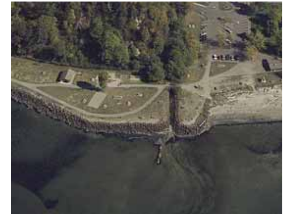
Shoreline armoring at mouth of McSorley Creek and along Puget Sound shoreline. See 1936 photo above left for comparison to historic shoreline location.
